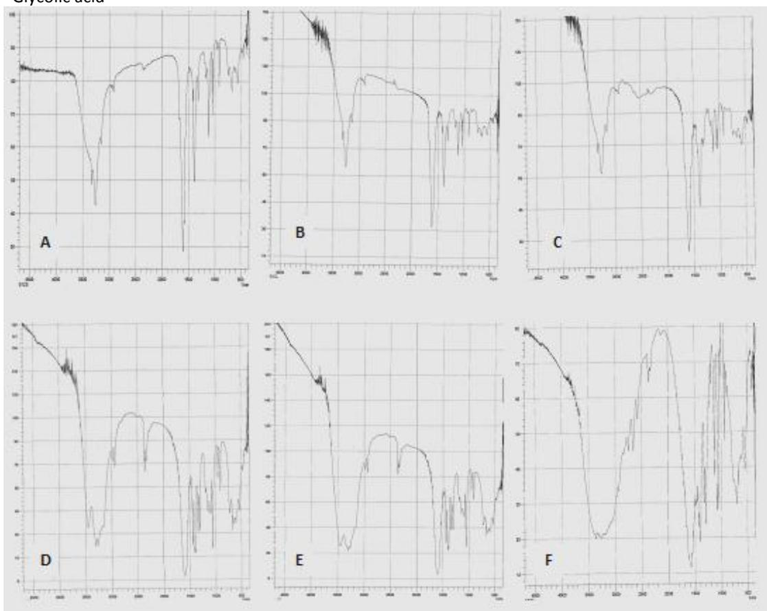
**Figure 1: IR spectra of (A) [Cu (L<sup>1</sup>)(Gly)], (B) [Cu (L<sup>2</sup>)(Gly)], (C) [Cu (L<sup>3</sup>)(Gly)], (D) [Zn (L<sup>1</sup>)( Gly)], (E) [Zn (L<sup>2</sup>)(Gly)], (F) [Zn (L<sup>3</sup>)(Gly)]**
