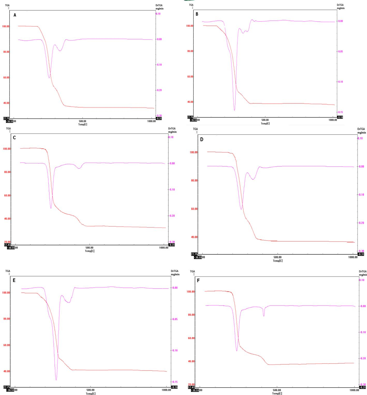
**Fig. 6 TG and DTG of ternary complexes: (A) [Cu (L<sup>1</sup>)(Gly)], (B) [Cu (L<sup>2</sup>)(Gly)], (C) [Cu (L<sup>3</sup>)(Gly)], (D) [Zn (L<sup>1</sup>)( Gly)], (E) [Zn (L<sup>2</sup>)(Gly)], (F) [Zn (L<sup>3</sup>)(Gly)]**
