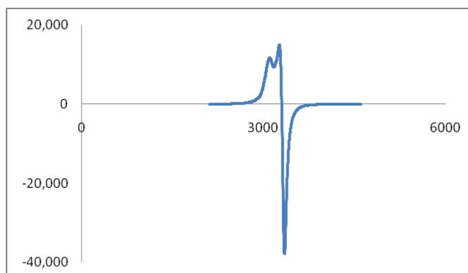
Figure 5: ESR spectra of [Cu (L<sup>3</sup>)(Gly)]
